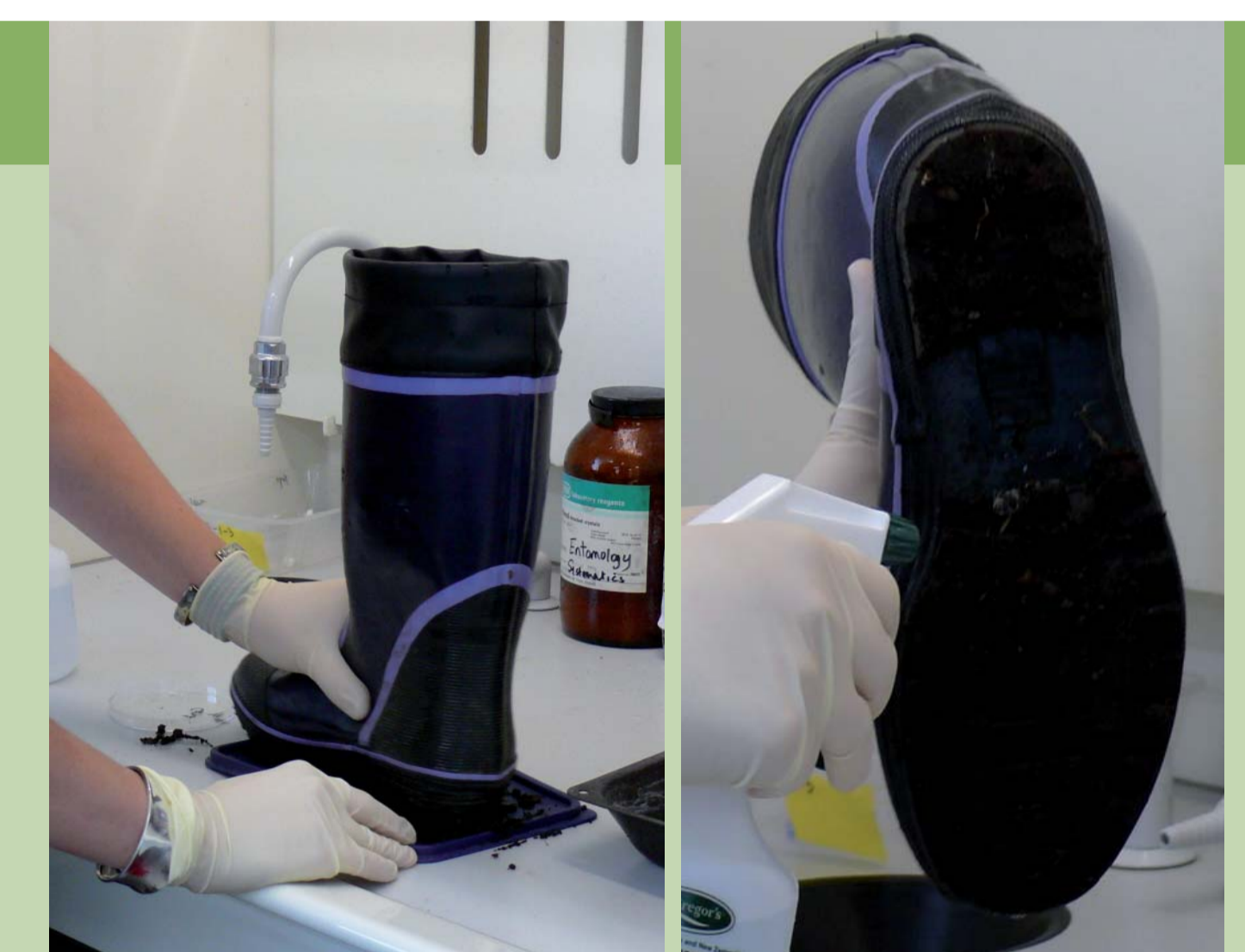
Figure 2 & 3: Rubber gumboot being pressed into soil "spiked" with PTA oospores (1,500 /g) and then sprayed with disinfectant to run-off
