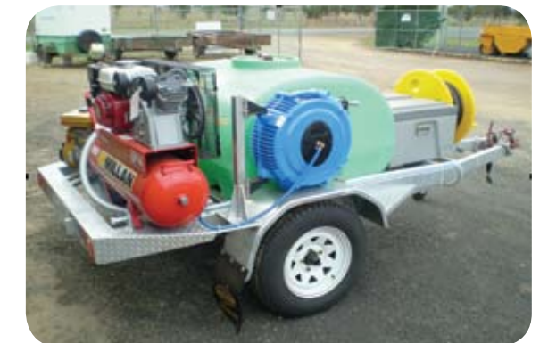
Mobile washdown unit with high pressure pump, hose and compressed air unit. Photo courtesy of NRM South/Southern Tasmanian Councils Authority.
