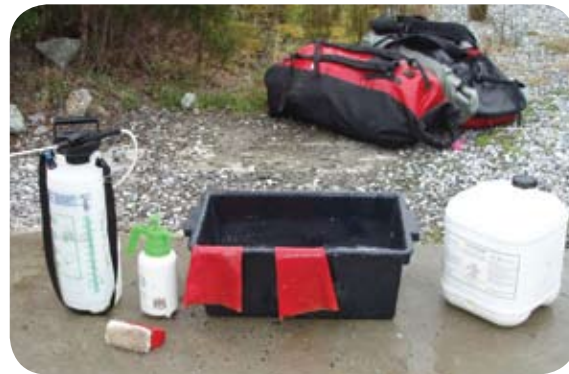
Field washdown equipment for simple field activities – spray bottles, footbaths, gloves, brush, disinfectant, measuring device. Photos courtesy of DPIPWE Water Assessment and Hydro Tasmania.
