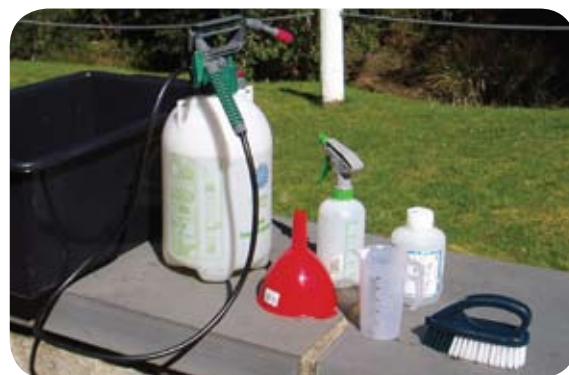
Field washdown equipment for simple field activities – spray bottles, footbaths, gloves, brush, disinfectant, measuring device. Photos courtesy of DPIPWE Water Assessment and Hydro Tasmania.
